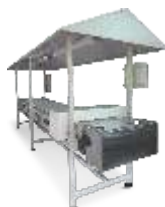
Inspection System & Metal Detector for cashew filling
